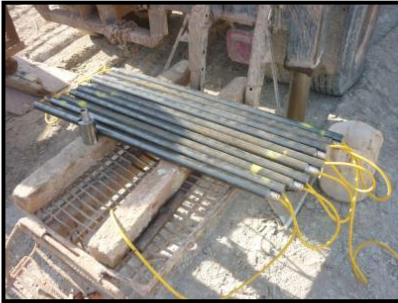
Figure (8): Geomil 10 cm 2 compression piezocone
