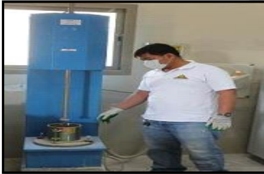
Figure (24): Laboratory compaction of soil using mechanical rammer (ASTM D-1557 and D-698))
