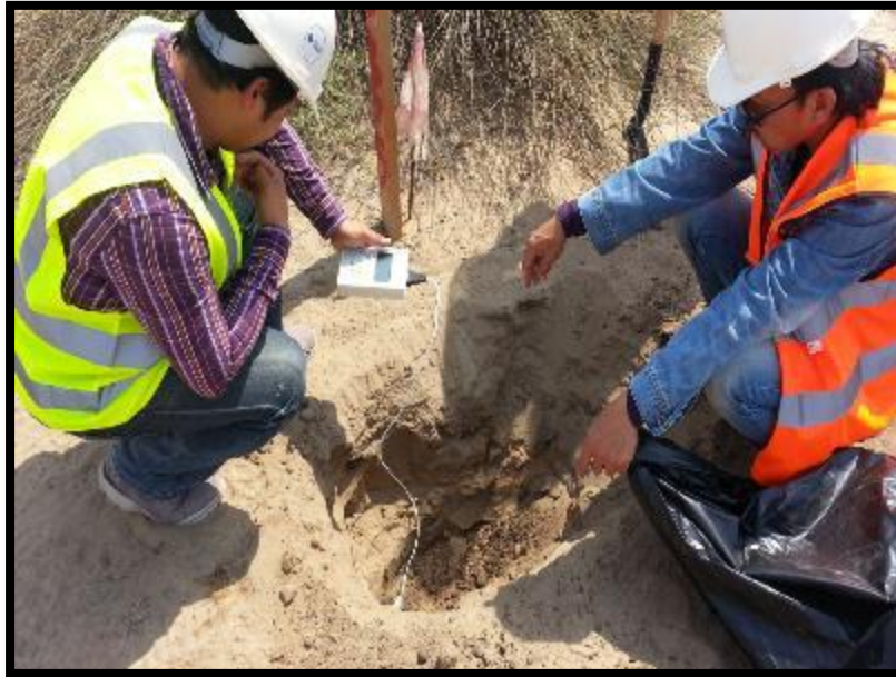
Figure (15): Thermal resistivity testing
