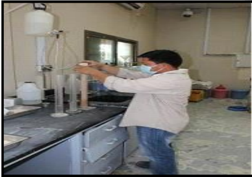
Figure (26): Sand Equivalent test (ASTM D-2419)
