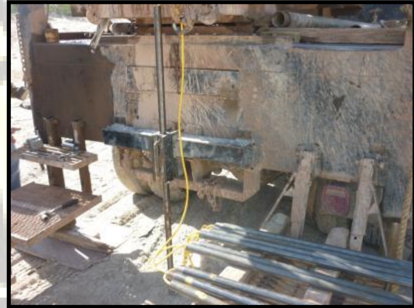
Figure (7): Geomil compression cone in operation
