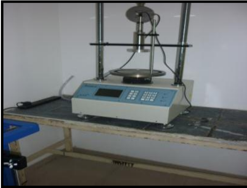
Figure (6): VJTECH Digital Triaxial Load Frame, 50 KN with Accessories
