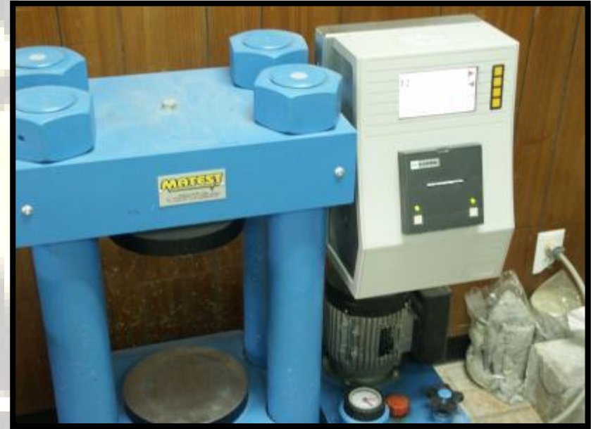
Figure (17): Concrete compression testing apparatus
