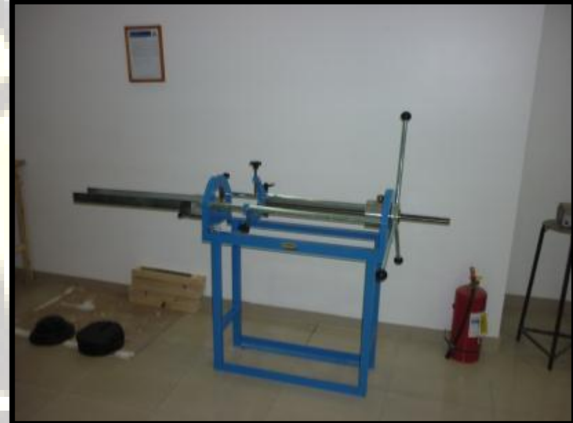
Figure (1): Soil Sample Extruder (Hand Operated)
