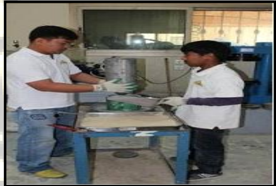
Figure (23): Minimum density determination of sand (ASTM D-4253)
