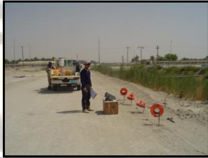
Figure (14): Field crew during electrical soil resistivity
