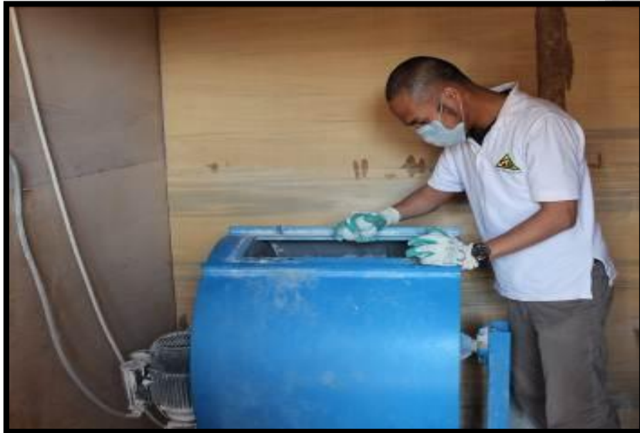
Figure (20): Abrasion of coarse aggregates by Los Angeles Machine (ASTM C-131)
