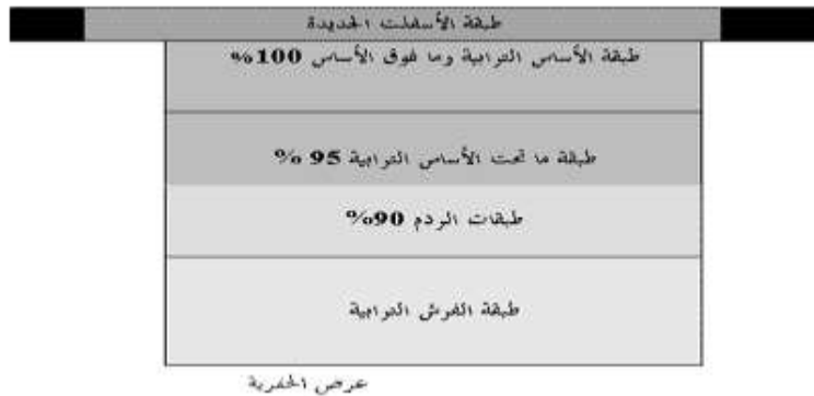
Specification of re-fill, asphalt cut and layer thickness layers - in the sub streets
