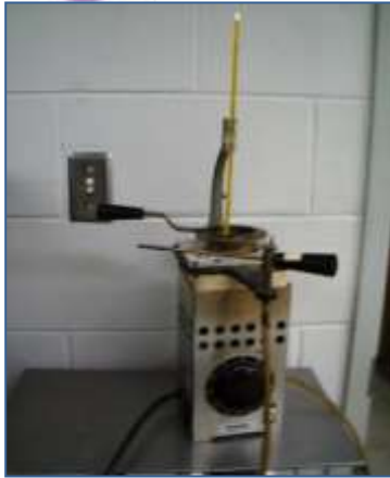
Flash and Fire point Test.
