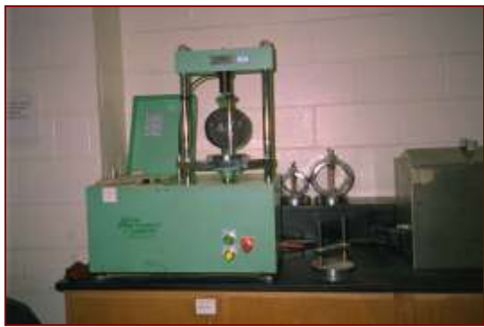
Marshall method - Stability test Pressure samples Marshall
