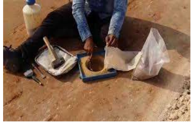
Soil density using the method (sand cone)
