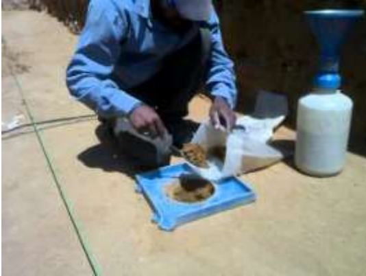
Soil density using the method (sand cone)
