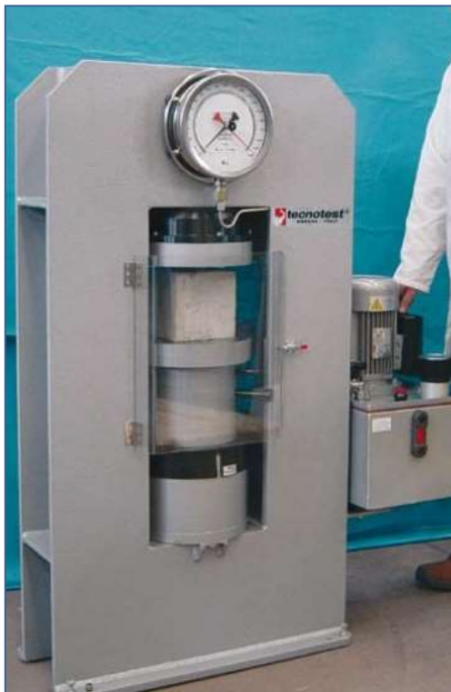
Mechanic Strength of Concrete by Compressive Strength test
